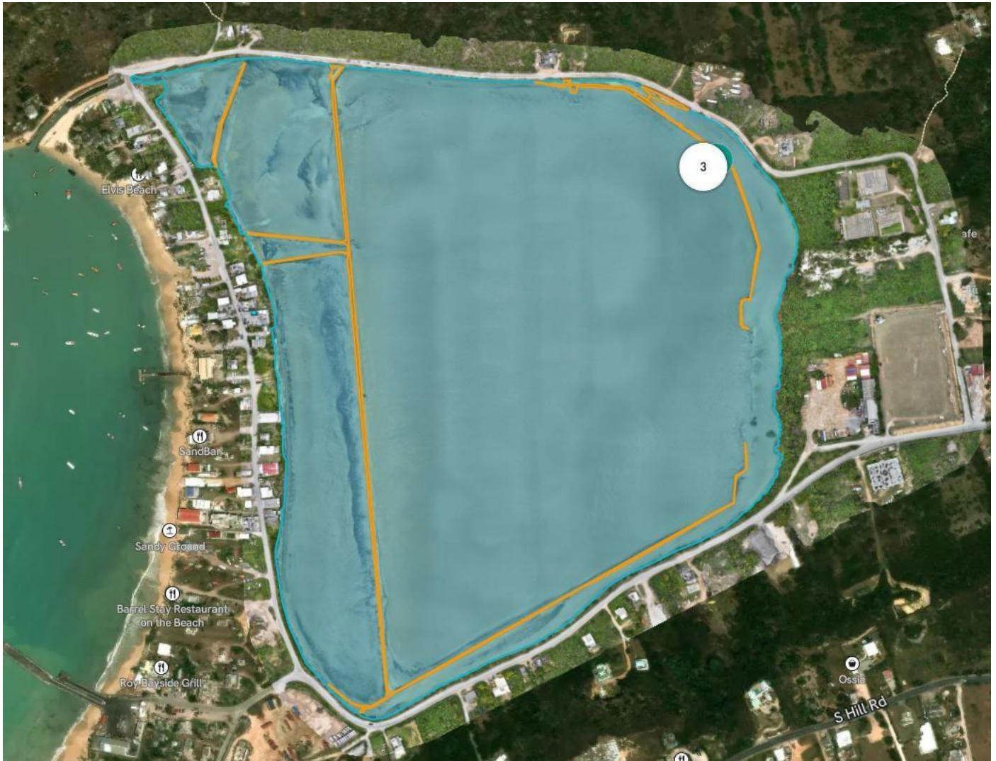
Figure 17. Annotated orthomosaic of Road Salt Pond showing key features including pond extent, earthwork dam structures, raft features, and georeferenced point data with elevation measurements for environmental monitoring.
