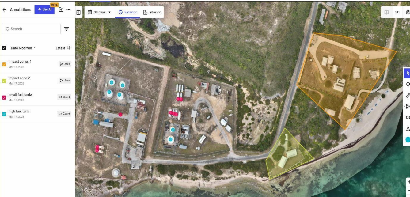
Figure 16. Annotated orthomosaic of Corito Bay derived from drone imagery, showing digitized fuel tanks, infrastructure, and impact zones for inspection and spatial analysis.
